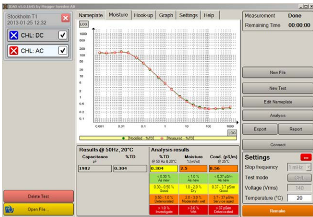
Fig. 4: Insulation assessment; Moisture, tan delta and oil conductivity
