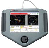
display permits the user to easily read all pertinent data while the test is being performed and provides the ability to view the current transformer's saturation curve. The unit can also be configured to come without a Megger STVI and can be controlled via a laptop with Megger's PowerDB software.
