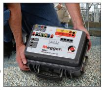
In addition the MRCT can be configured to test kneepoints up to 30 kV using an alternative DC technique. This allows testing the majority of CTs using line frequency while still being able to test larger generation class CT with a portable instrument.
